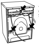
You must remove the shipping supports before you install the washer.
